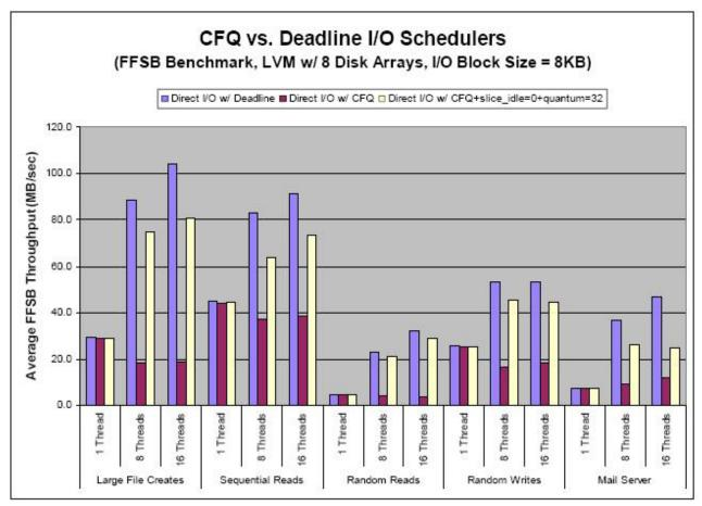
The figure shows the average FFSB throughput in megabytes per second for direct I/O paired with the following types of I/O schedulers:
