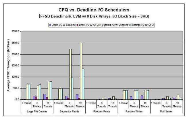
The figure shows the average FFSB throughput in megabytes per second for each type of I/O paired with each type of I/O scheduler as follows:
