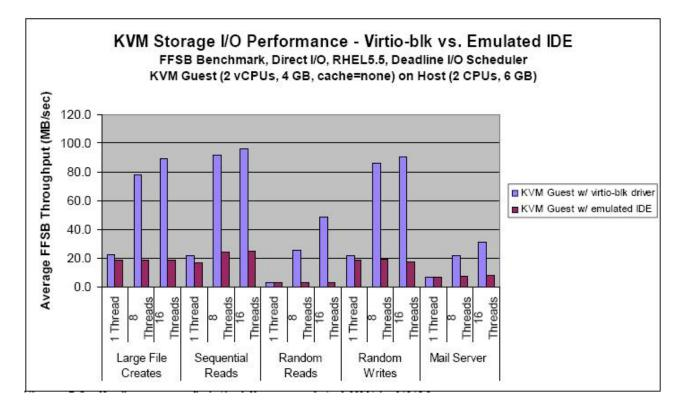
The figure shows the average FFSB throughput in megabytes per second for the guest operating system run with a virtio\_blk driver and the guest operating system run with an emulated IDE device. For both the virtio\_blk driver and the emulated IDE device, the figure shows throughput data for the following types of operations:
