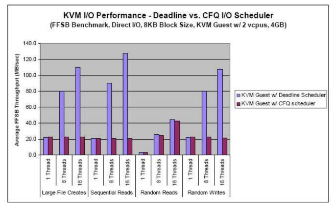
The figure shows the average FFSB throughput in megabytes per second for the guest operating system run with the Deadline I/O scheduler and for the guest operating system run with the CFQ I/O scheduler. For each I/O scheduler, the figure shows throughput data for the following types of operations:
